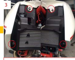
▲ Remove the 4 bolts in front of the fuel tank cover
