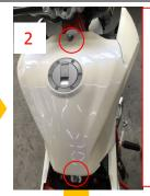
Remove the two bolts on the tank
