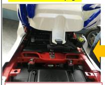
▲ Lift the tank and put the battery in and install the battery strap
