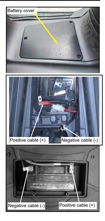
Install the battery in reverse order of removal.
