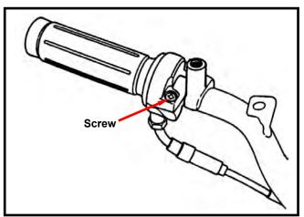
Remove the rear brake lever nut and screw, Remove the brake seat bolt, and then remove the seat.
