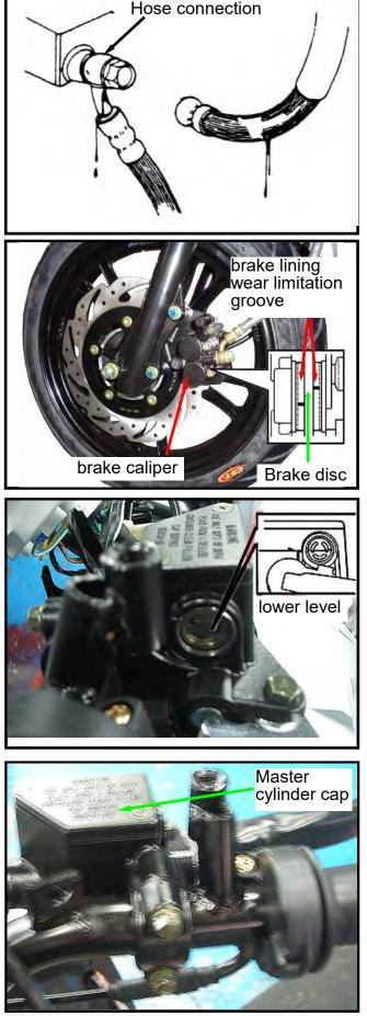
Remove the master cylinder cap and diaphragm.
