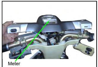
Remove the front cover. Remove the power connector of the meter.
