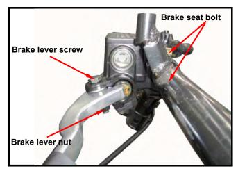
With a wrench to hold the handlebar bolt and then remove the nut. Take out the handlebar after removed the bolt.
