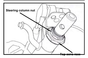
With a plastic hammer to tap the steering column slightly, and then remove the top ball bearing seat.
