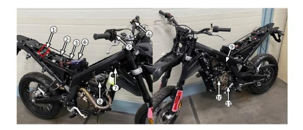
1 start relay/auxiliary relay, 2 ECU, 3 fuse box, 4 battery, 5 right combination switch,
