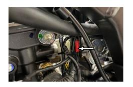
Remove the ignition coil spark plug cap.
