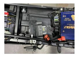
3. Loosen the fastening screws of the air cleaner cover and take out the air cleaner cover
