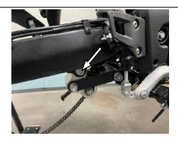
5. Loosen the flat fork shaft nut and pull out the flat fork shaft from the left side to pull out the flat fork backward.
