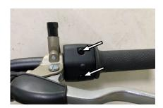
4. Remove the fixing screw of throttle cable.
