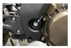
Disassemble the gearshift subassembly and remove the left rear cover, and remove the drive chain
