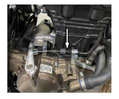
Remove the output line, gear display line and switch line of the magneto.
