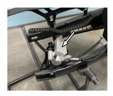
4. Remove the rear shock absorber and flat fork connecting bolt M10×(38+16).
