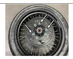
8. Take out the disc of rear disc brake.
