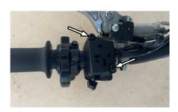
7. Remove the left combined switch screw.
