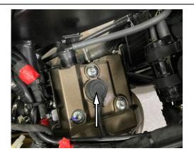
Remove the spark plug and test the cylinder pressure
