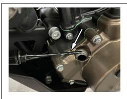
Replenish method: pull off the filler cap of the accumulator, and use the funnel to guide the coolant slowly until the coolant level is at the upper limit of the middle part. Then cover the water filler cap.
