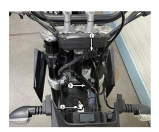
1. Instrument wiring, 2. Front turn signal wiring, 3. Headlamp wiring
