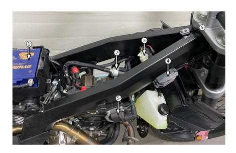
1 Battery, 2 Fuel filter, 3 Handle switch wiring, 4 Voltage regulating rectifier, 5 Ignition coil
