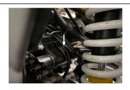
The engine number is printed on the right side of the crankcase, near the rear shock absorber. The engine number can be seen from the rear right side of the vehicle.
