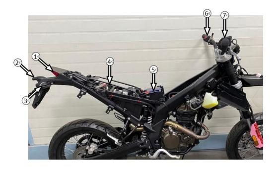
1 Combined tail lamp, 2 License plate lamp, 3 Rear right turn signal lamp, 4 Flasher, 5 Battery, 6 Left combination switch, 7 Right combination switch
