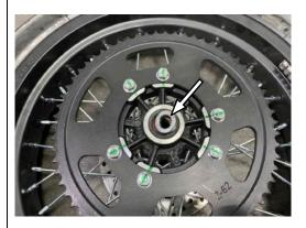
7. 7. Remove the six M8×30 fastening bolts of the chain wheel and take out the chain wheel to get the rear wheel.
