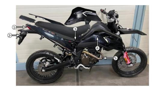
1 Tail light component, 2 Rear fender, 3 Frame, 4 Closure panel, 5 Muffler
