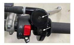
8. Remove the handlebar clip fixing bolt.
