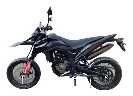
Except for the positions shown in the figure above, except that the special engine oil for the chain is used for the drive chain, lithium base grease is used for other positions.
