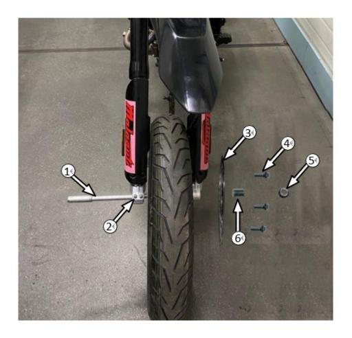
1 Front axle, 2 Front axle fastening bolts, 3 Front brake disc, 4 Front brake disc bolts, 5 Front axle nuts, 6 Front wheel left bushing
