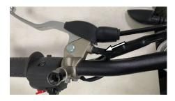
2. Remove the front brake master cylinder clip bolt.
