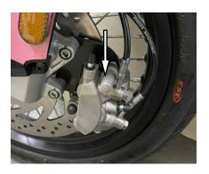
Front brake caliper body
