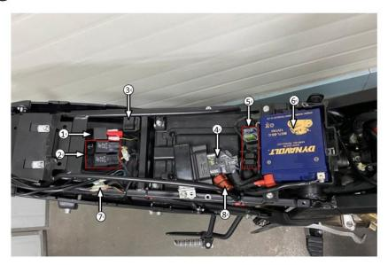
1 Start relay, 2 Auxiliary relay, 3 Flasher, 4 ECU, 5 Fuse box, 6 Battery, 7 Tail lamp rear turn signal wiring, 8 OBD interface
