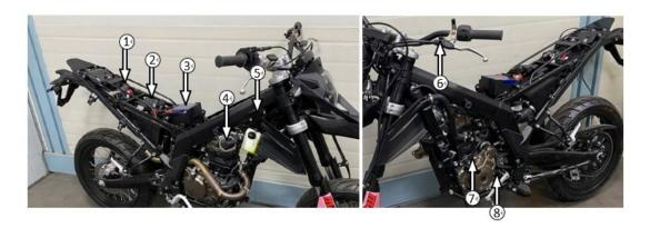
1 Start relay, 2 ECU, 3 Battery, 4 Ignition coil, 5 Rectifier,6 Clutch switch, 7 Magneto harness, 8 Gear switch
