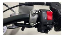
6. Remove the clutch handle bolt.
