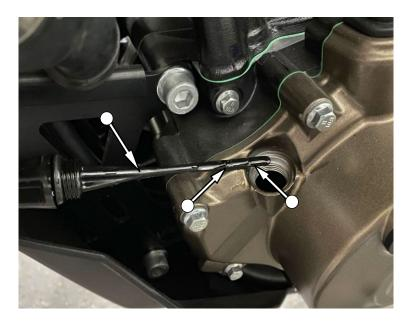
1 Oil level gauge, 2 Upper limit line of oil level gauge, 3 Lower limit line of oil level gauge
