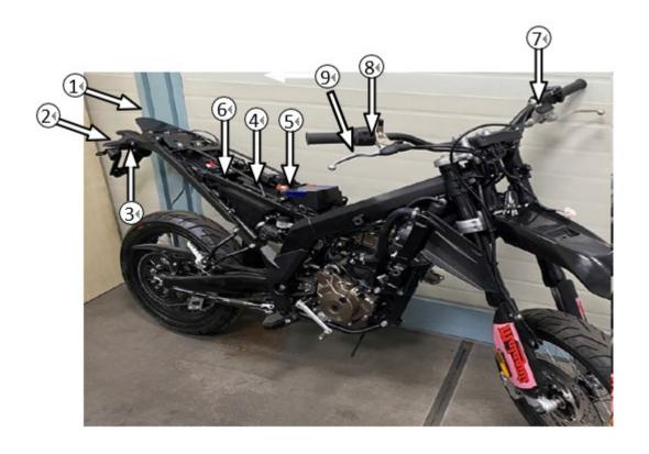
1 Combined tail lamp, 2 License plate lamp, 3 Rear right turn signal lamp, 4 ECU, 5 Battery,
