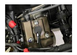
Remove 4 bolts of M10×100 from the front of the engine cradle to the frame, 2 bolts of M10×25 from the top to the frame, and the rear fork to the frame connecting shaft.
