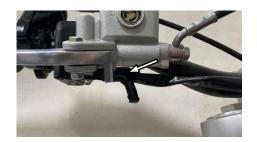
5. Pull off the clutch switch plug.
