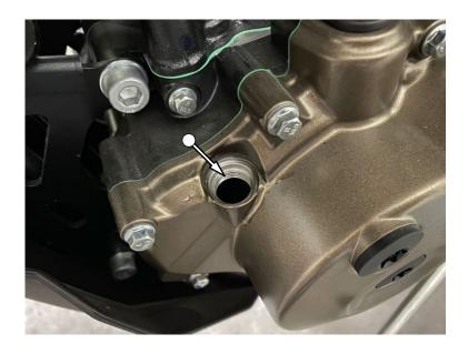
1 Loosen the oil drain bolt, 2 Oil filling port
