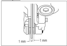
The brake pads must be checked at regular intervals. In the best case, before every journey. The pads have a notch that must always be visible. The wear of the pads depends on the driving style and the road surface. When the minimum pad thickness of 1 mm is reached, both pads must be replaced. Leave the replacement of the brake pads to the specialist dealer. Worn brake pads increase the braking distance.
