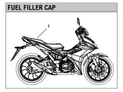
The fuel filler cap (1) is located under the seat.
