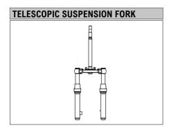
The condition of the telescopic suspension fork must be checked according to the maintenance table. Furthermore, it should be briefly checked before each ride and treated with care products if necessary.
