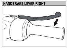
The brake lever for the front brake is located on the handlebar on the right. To brake, pull the lever towards the handlebar.
