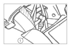
Unscrew the spark plug with the spark plug spanner (2) of the on-board tool.
