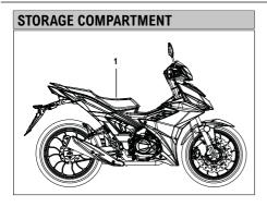
The storage compartment (1) is located under the seat.
