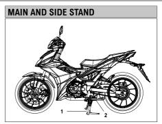
The side stand (1) is located on the left side of the vehicle. Unfold the side stand with your foot and park the vehicle.
