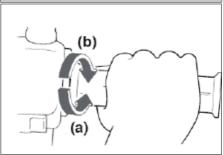
The speed is also controlled with the throttle grip.
