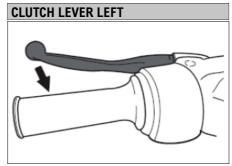
The lever for operating the clutch is located on the handlebar on the left. To engage the clutch, pull the lever towards the handlehar
