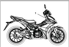
The USB charging port (1) is located under the handlebar.
