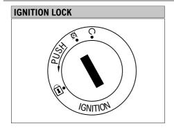
The ignition lock controls the ignition and lighting system and is used to lock the steering and open the seat. The positions are described below.
