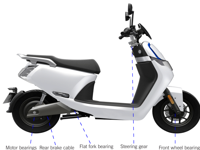
Lubrication parts of MOTRON WHIZZ electric vehicle
