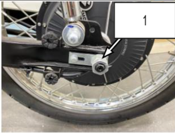
1) Rear axle fastening nut
