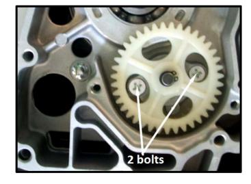
Install oil pump outer cover (2 bolts).
