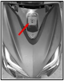
Remove the mounting screws and bolt.
