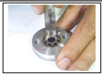
Check clearance between inner and outer rotors.
