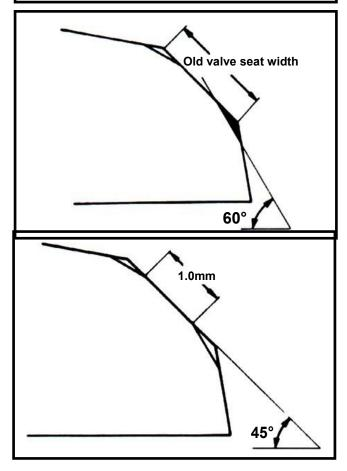
Coat the valve seat surface with red paint. Install the valve through valve guide until the valve contacting with valve seat, slightly press down the valve but do not rotate it so that a seal track will be created on contact surface.
