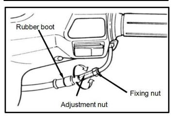
Primary adjustment is conducted from button side. Loosen fixing nut, and adjust by turning the adjustment nut.
