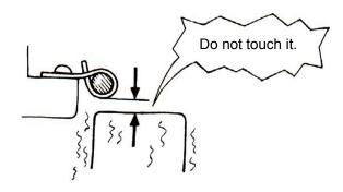
Route wire harness to avoid sharp edges or corners and also avoid the projected ends of bolts and screws.
