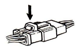
Do not pull the wires as removing a connector or wires. Hold the connector body.
