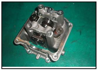
After removed valve cotters, release the compressor and then take out spring retainer, valve spring and valves.
