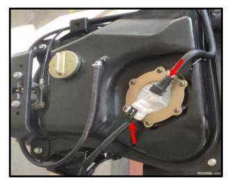
Remove the fuel pump lock bolts.
