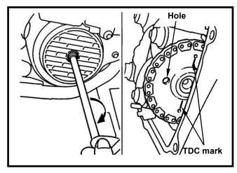
Remove camshaft holder nut and washer.
