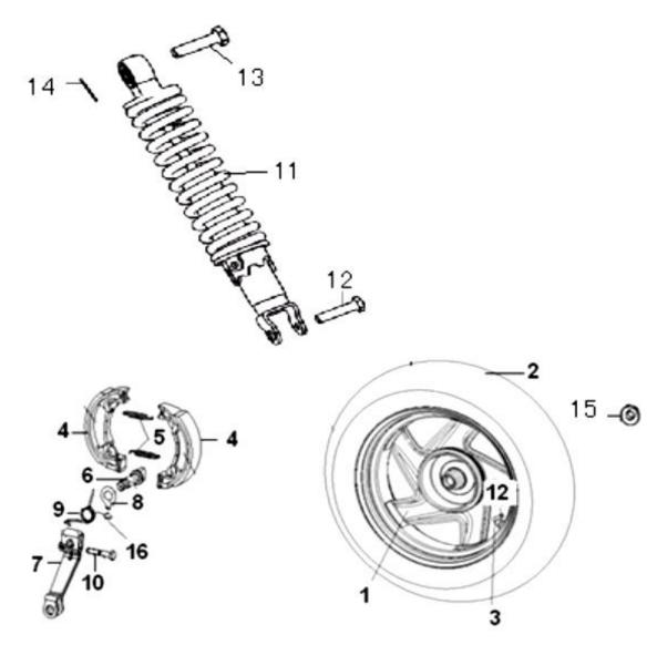
1 RR. RIM COMP. 3.5X12 2. TIRE 120/70-12 3. RIM VALVE Z2-01-1 4. BRAKE SHOE KIT 5. SPRING(BLACK) 6. CAM SHAFT 7. CAM SHAFT LEVER, ASSY 8. BRAKE INDICATOR PLATE 9.TENSION SPRING 10. HEX. BOLT 6X30MM 11. RR. ABSORBER ASSY. (BLACK) 12. BOLT (GOLD COLORED)8X31MM 13. BOLT10X1.25 X40MM 14. SPLIT PIN (GOLD COLORED)1.2X22MM 15. U NUT 16X1.5MM
