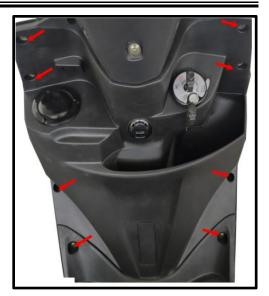
Remove the front under cover 2 mounting screws Between the front under cover and the frame.
