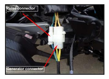
Remove the 6 bolts for the pulse generator, the A.C. generator coil and cable guide. Then, remove the A.C. generator assembly.
