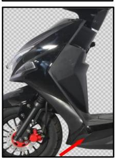
Remove the mounting screws and bolt.(8 screw)
