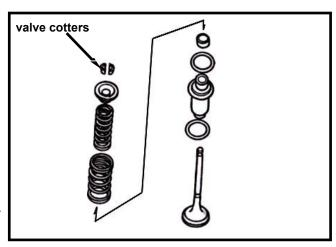
Remove valve stem guide seal.
