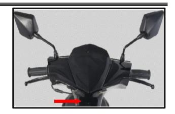
Remove the front handle cover. Remove the speedometer cable.
