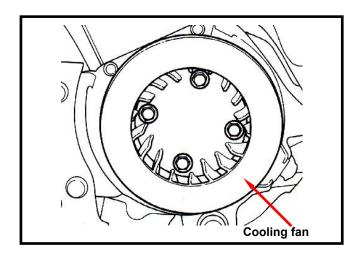
Install the cooling fan shroud. (4 bolts)
