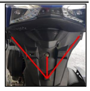
Remove the 2 mounting screws the Battery cover.
