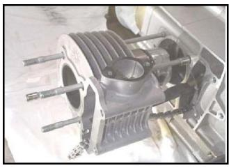
Remove cylinder gasket and lock pins
