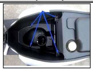
Disconnect the fuel pump couplers. Disconnect the fuel unit couplers Remove the fuel pipes.
