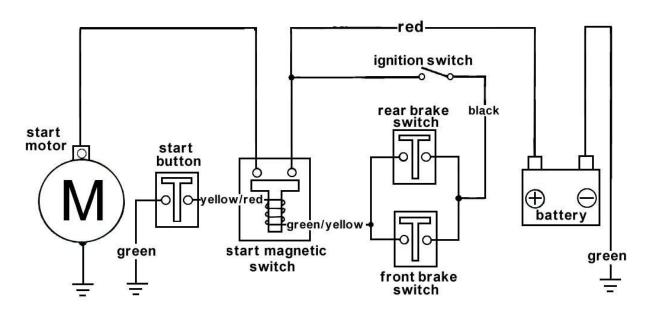
Starter magnetic switch inspection Turn main switch to "on", and operate the brake lever. Then press starting button to check if there a click sound. It is normal if there is a click sound.
