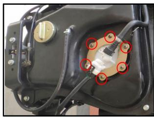
Remove the fuel pump and fuel unit.
