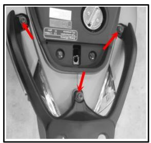
Remove the 2 mounting bolts of the rear fender.
