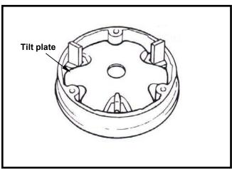
Remove weight rollers from sliding pulley.
