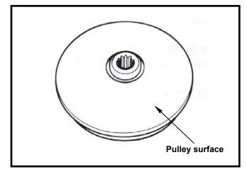
Install siding pulley assembly onto crankshaft.
