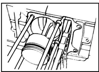
Clean the residues attached onto the matching surfaces of cylinder and crankcase.
