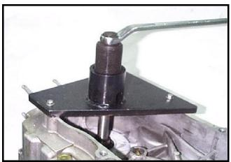
Remove the crankshaft from the right crankcase.
