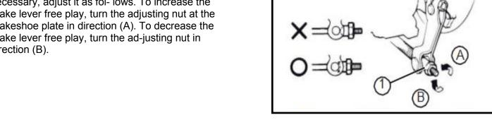
Always check and adjust the brake lever before riding. To check the bra-ke, check the position of the adjustab- le nut if the nut position reach to the end, have a dealer to replace the brake shoes as a set.
