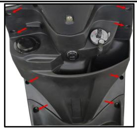
Remove the hook screw bolt from the Top of toolbox .
