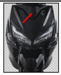
Remove the mounting screws and bolt.
