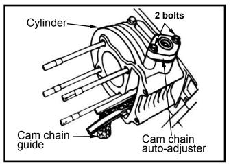
Remove cam chain plate. Remove cylinder.
