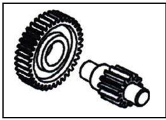
Check if the final driving shaft and gear are burn, wear or damage.
