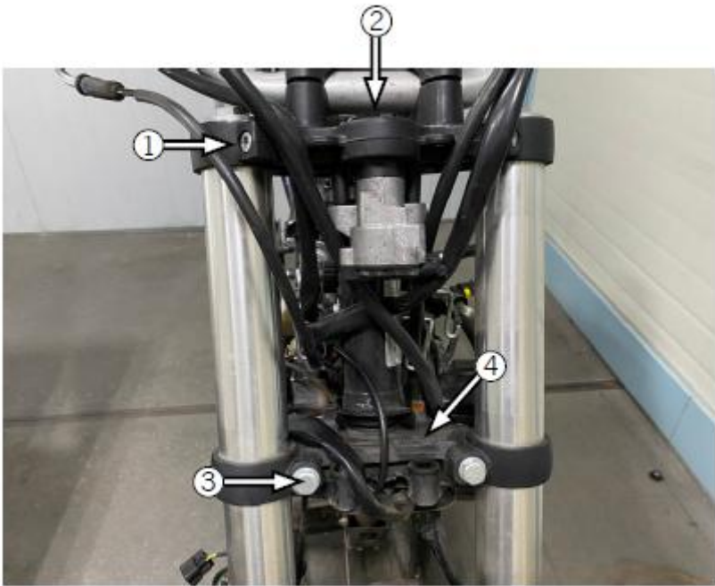
1 Upper damping bolt, 2 Steering column locking bolt, 3 Lower damping bolt, 4 Steering column combination
