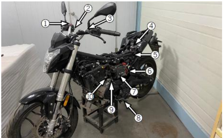
1 Flameout switch, 2 Start switch, 3 Clutch switch, 4 ECU, 5 Cable harness, 6 Start relay, 7 Battery, 8 Side bracket switch, 9 Gear switch, 10 Start motor
