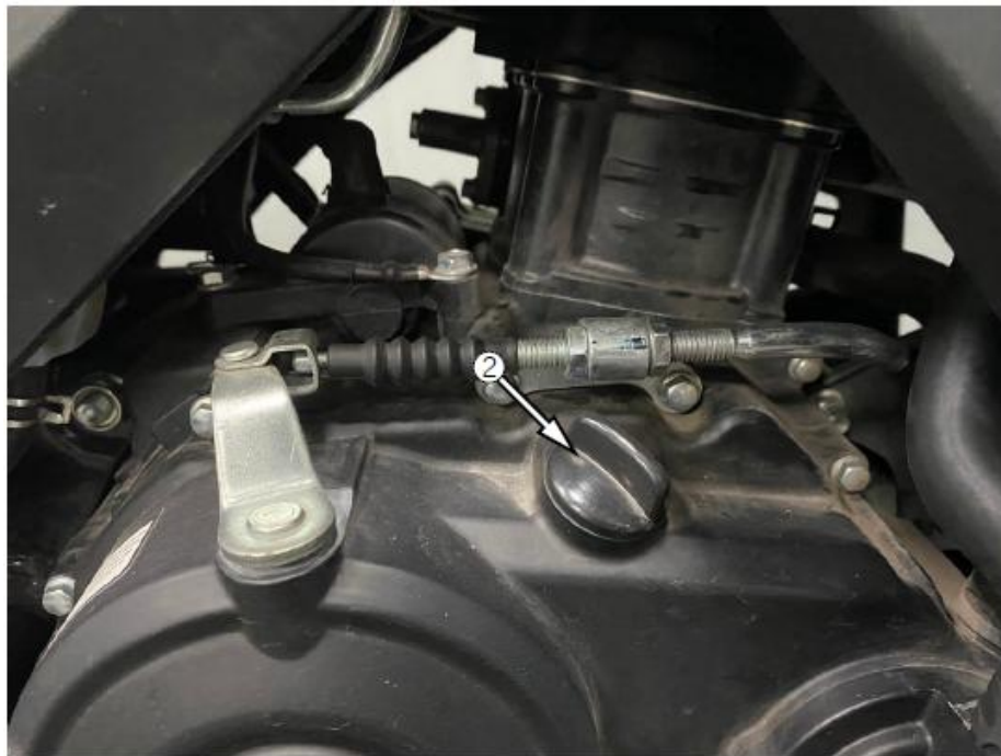
1 loosen the oil drain bolt and 2 fill the oil
